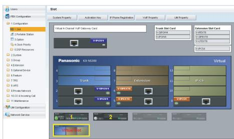
1. Click **Setup** → **PBX Configuration** → **Configuration** → **Slot**.
