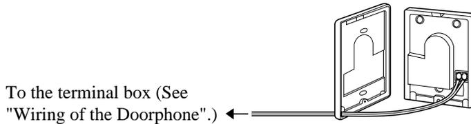
4. Secure both halves together and re-install the screw.
