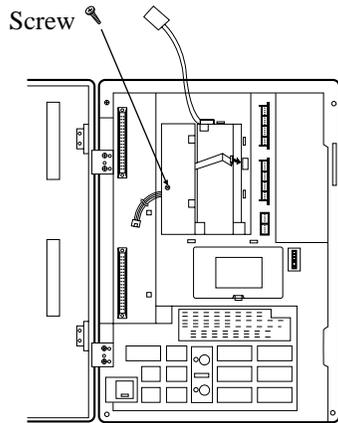
4. Connect the cord of battery to the adaptor card. Remove the backup battery connector cover on the main unit. Then connect the cord of the adaptor card to the backup battery connector.
