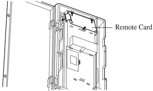
2. Press down the two corners of the lower side of the Remote Card.
