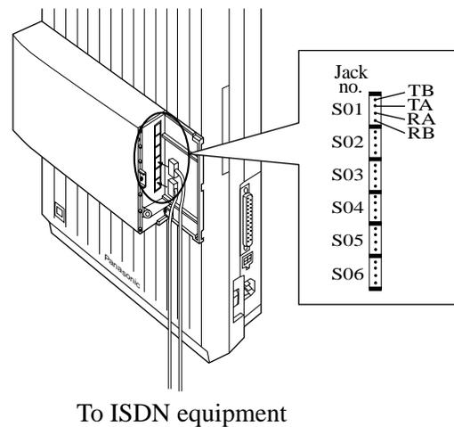
3. Connect the lines between the ISDN board and the ISDN device.
