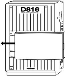
**Installing the DISA Card (KX-TD199) to the Remote Unit (KX-TD198) /
