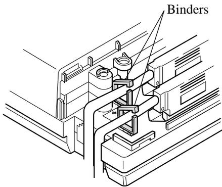
3. If two units are connected with the DC IN/OUT or a Battery Adaptor (KX-A46) is connected to the unit, insert the 4-pin connectors to the jacks as shown below. Also connect the ground terminal of the unit to the minus (-) terminal of a car battery using an earth wire.
