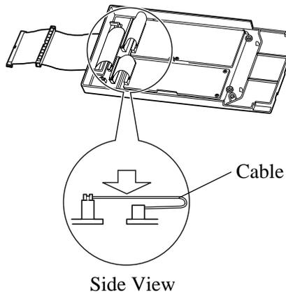
6. Replace the inside cover and secure the four screws on the back. Also, replace the side cover.
