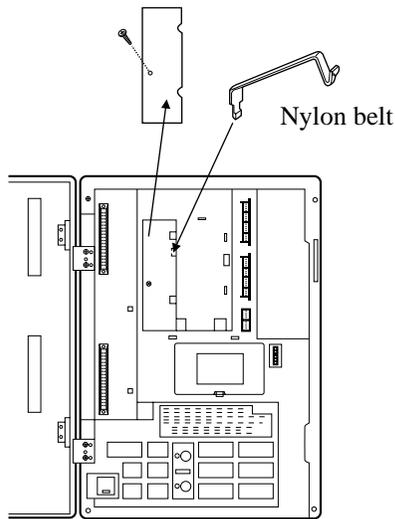
2. Insert the battery and adaptor card into the frame.\*<sup>2</sup>
