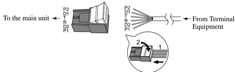
2. Insert the plug into an extension jack in the main unit.
