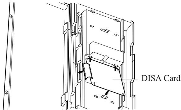
**2.** Press down the two corners of the lower side of the DISA Card.
