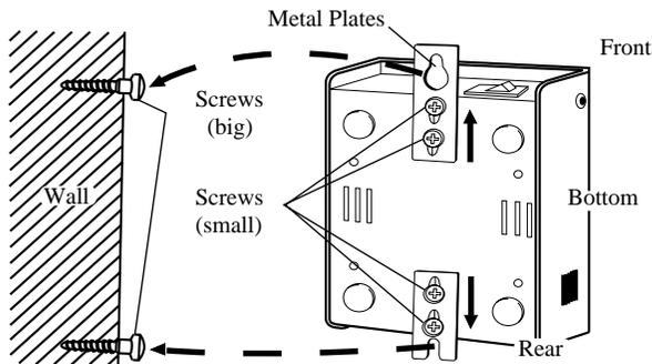
**Mounting on Concrete or Mortar Walls;**
