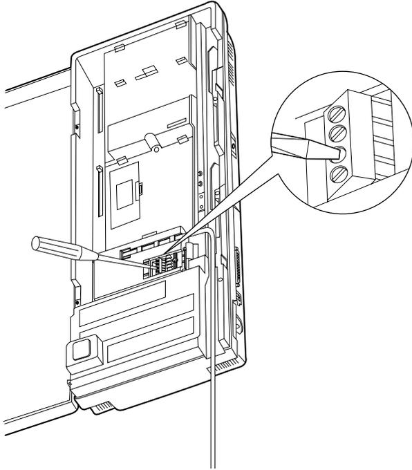
3. Insert the wires coming from the door openers into holes and tighten the screws.
