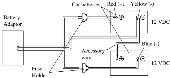
2. Insert the plug of the battery adaptor into the battery adaptor connector on the main unit.
