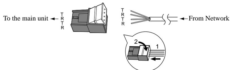
2. Insert the plug into an outside line jack in the main unit.
