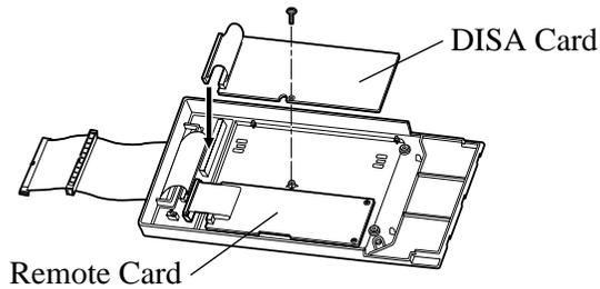
5. Flatten the cable to replace the inside cover properly.
