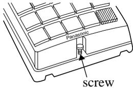
2. Install the base cover to the wall with two screws.
