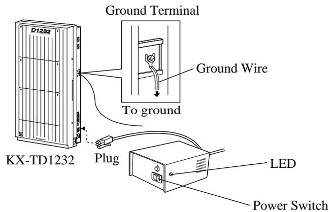
3. Turn on the power switch of the battery adaptor.
