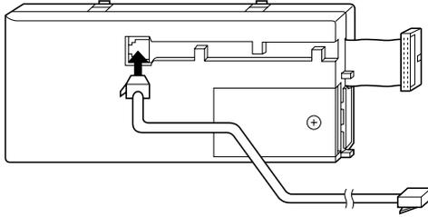
2. Attach the Doorphone Card Cabinet to the main unit and press down.
