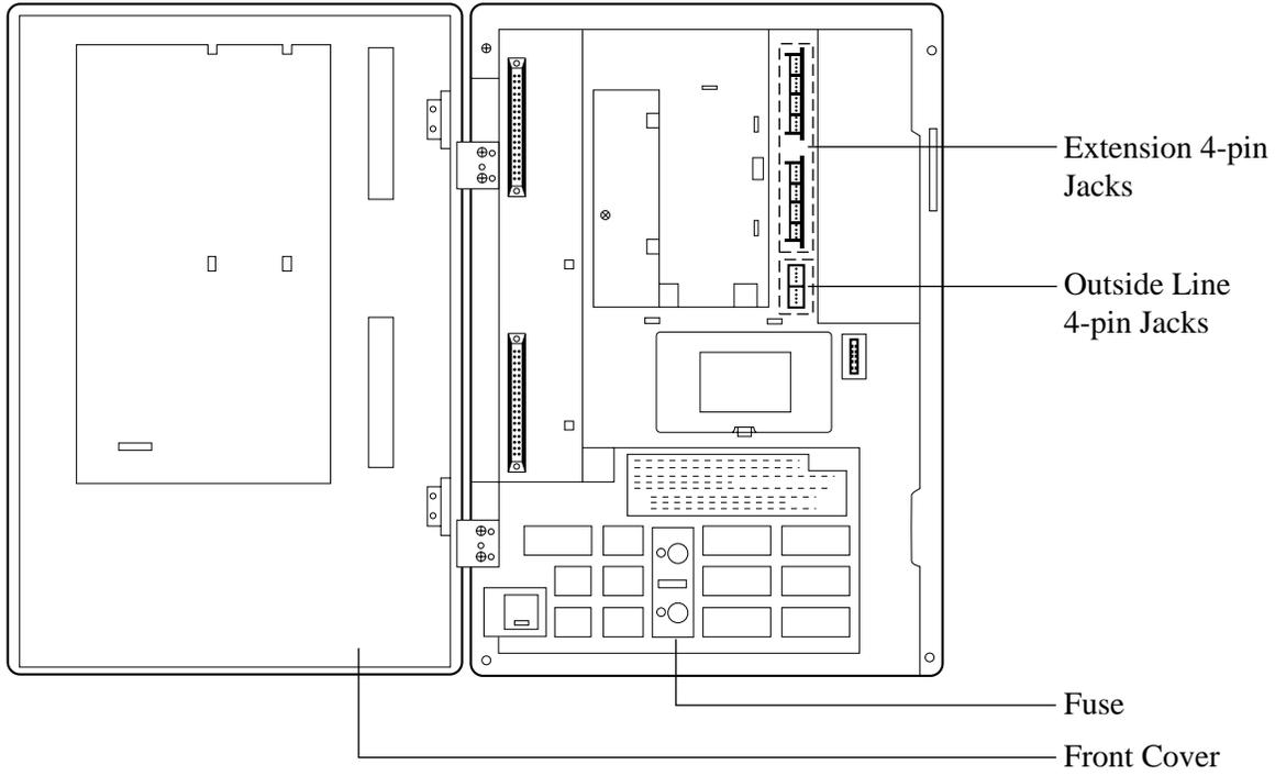
**KX-TD1232 (4-pin / 6-pin Connector Type)**
