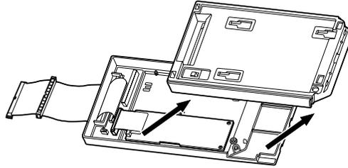
4. Install the card, secure the screw (included with the unit) and connect the cable to the connector.
