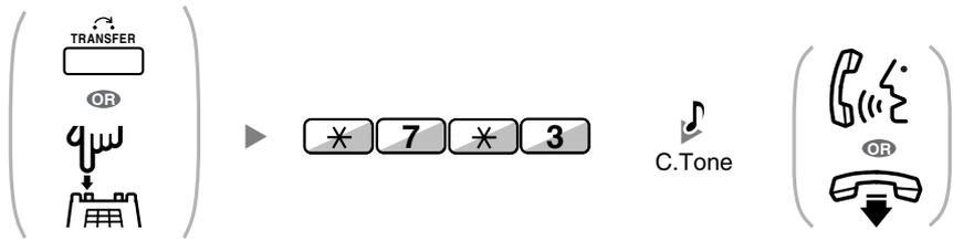
The diagram illustrates the process of requesting Malicious Call Identification (MCID). It is divided into three main stages:
