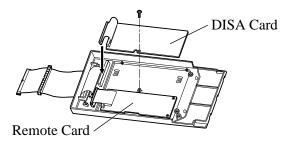
**5.** Flatten the cable to replace the inside cover properly.
