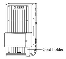
10.Fix the cords to the wall as shown so that the front cover can be opened.
