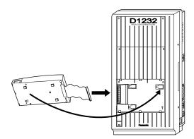
**3.** Hook the cabinet to the main unit and slide the cabinet to the left until it is secured.
