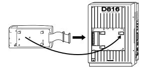
**3.** Hook the cabinet onto the main unit and slide the cabinet to the left until it is secured.
