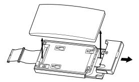
**2.** Turn over the unit and remove the four screws.
