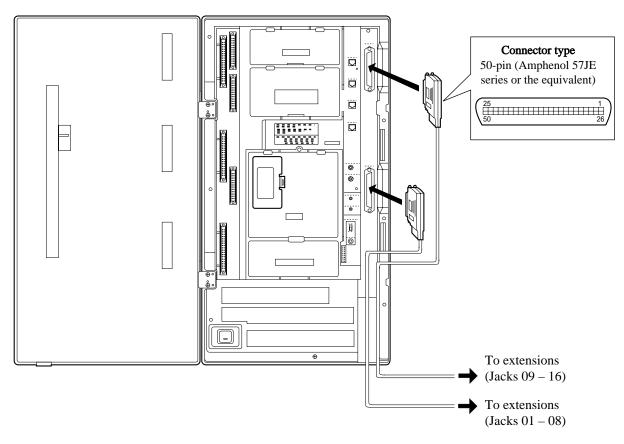
**3.** After inserting the connector, fasten the connector with the nylon tie.
