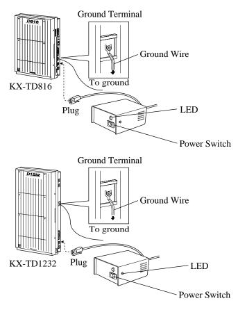
**3.** Turn on the power switch of the battery adaptor.
