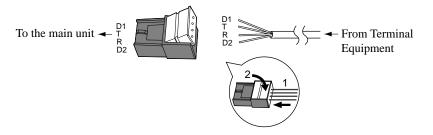
2. Insert the plug into an extension jack in the main unit.
