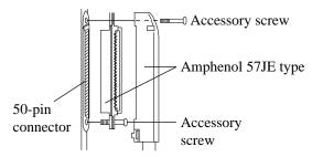
**2.** To attach the Amphenol 57JE type (Plug) to the connector, drive the accessory screw into the upper part.
