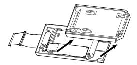
**4.** Install the card, secure the screw (included with the unit) and connect the cable to the connector.
