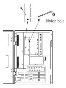
2. Insert the battery and adaptor card into the frame.\*2
