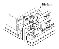
**3.** If two units are connected with the DC IN/OUT or a Battery Adaptor (KX-A46) is connected to the unit, insert the 4-pin connectors to the jacks as shown below. Also connect the ground terminal of the unit to the minus (-) terminal of a car battery using an earth wire.
