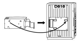
4. Hook the cabinets onto the main unit and slide the cabinets to the left until they are secured.
