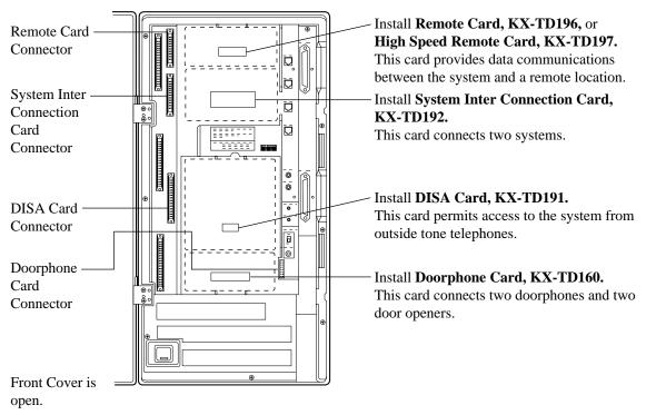
Remote Card, System Inter Connection Card, DISA Card, Doorphone Card for KX-TD1232
