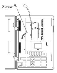
**4.** Connect the cord of battery to the adaptor card. Remove the backup battery connector cover on the main unit. Then connect the cord of the adaptor card to the backup battery connector.
