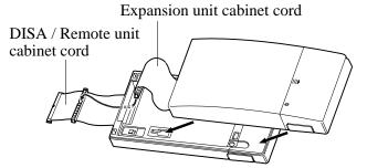
**3.** Remove the cover plate and connect the cabinet cord to the connector in the main unit firmly.
