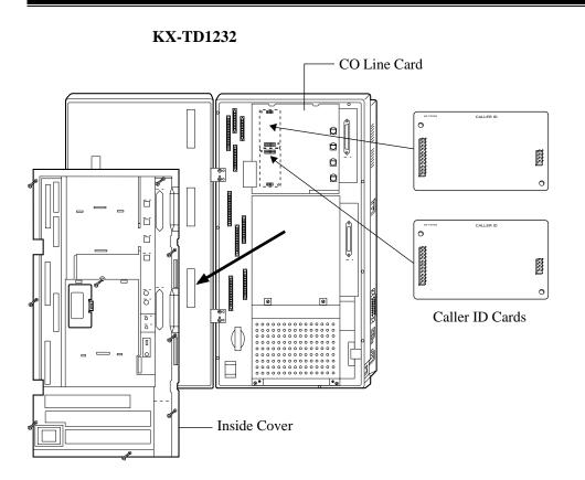
**3.** Put the inside cover back on the main unit and secure the screws.
