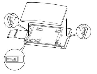
**2.** Attach the expansion unit to the DISA or Remote Unit as shown below. Be sure to connect the cabinet cords by inserting the expansion unit cabinet cord through the slot in the DISA or Remote Unit.
